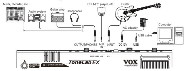
Set the AMP/LINE switch appropriately for the type of device you'll be connecting to the OUTPUT/PHONES jack.
