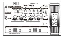
2. Press the AMPS bank select switch to select a bank, and use the AMPS/STAND ALONE PEDALS selector to select an amp model.
